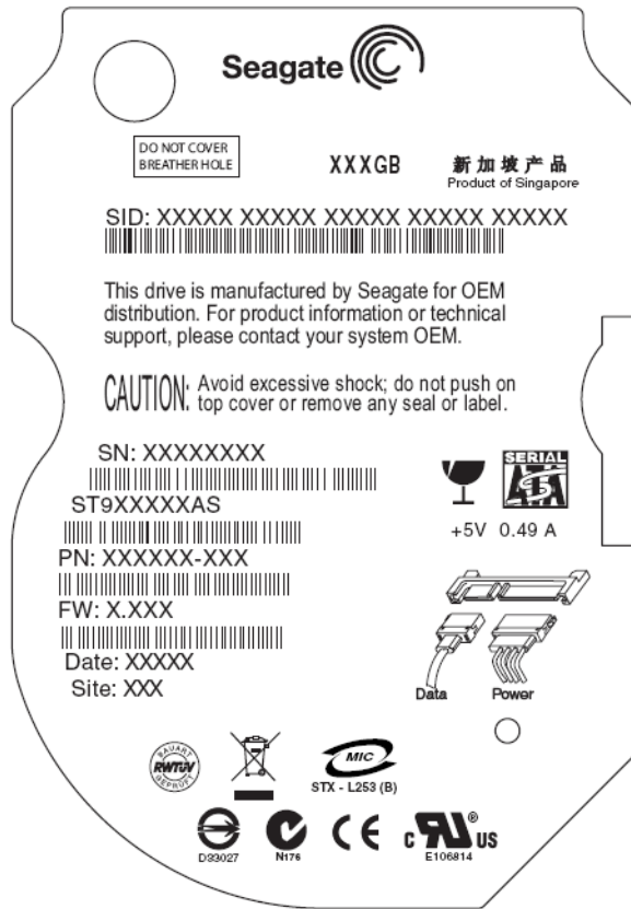
Figure 5. Momentum 5400 FDE.4 SATA drive label example
